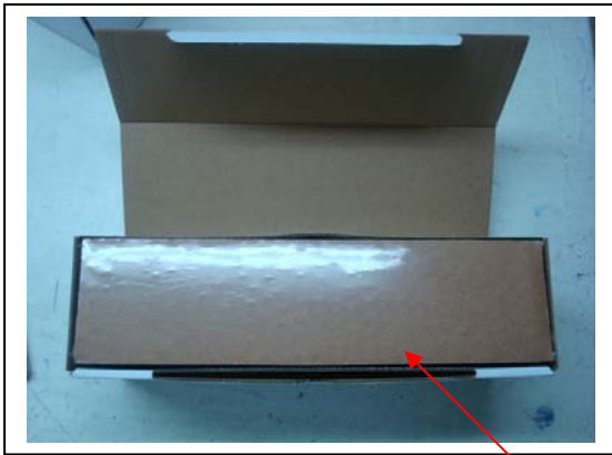
The corrugated board with plastic sealed.
